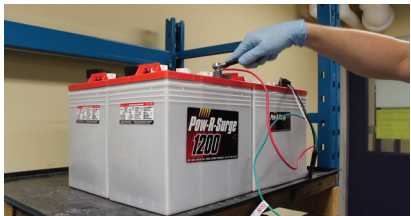
Figure 2: Remove positive lead from positive terminal on the battery pack.
