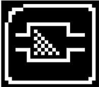
**Fuel Filter** - Diesel filter is changed. This filter is important to the general efficiency of diesel engines. As the fuel passes through this filter, unwanted particles and residue will become trapped, so that the fuel is passing to the engine is 'clean'. Therefore, this filter has to be replaced when indicated to ensure that your engine is running at optimum performance.
