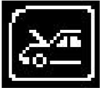
Diagnostic / Vehicle Selection Icon – Select this to go into Vehicle Specific Serial Diagnostics
