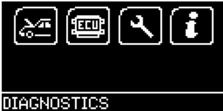
Connect the EQP-061 Tool to a vehicle using the 16 Pin Diagnostic plug. The EQP-061 Tool will then power up and take you to the Main Menu screen.
