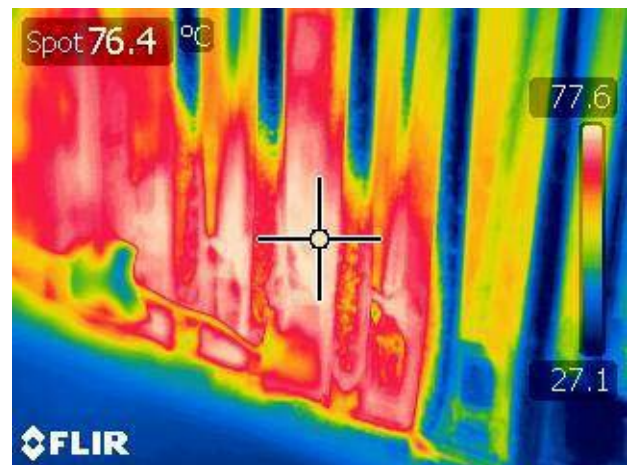
Figure 10. IC650 left side. The highest measured temperature in this area is 77°C (170°F).
