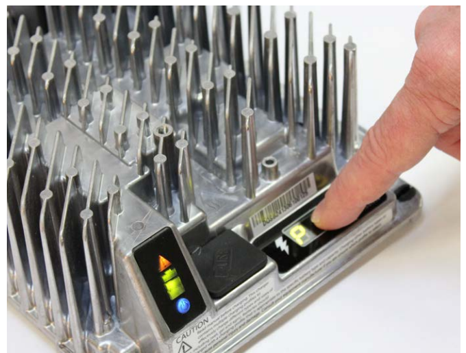
Figure 27. Press the Select Charge Profile Button to advance through the charge profiles. When the desired charge profile appears, hold the button for 10 seconds to confirm your selection.
