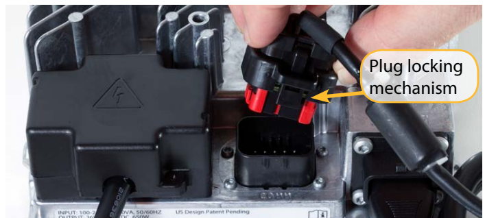
Figure 20. Insert the TE Connectivity AmpSeal Plug into the Comm fixture with the locking mechanism facing toward the outer edge of the charger.
