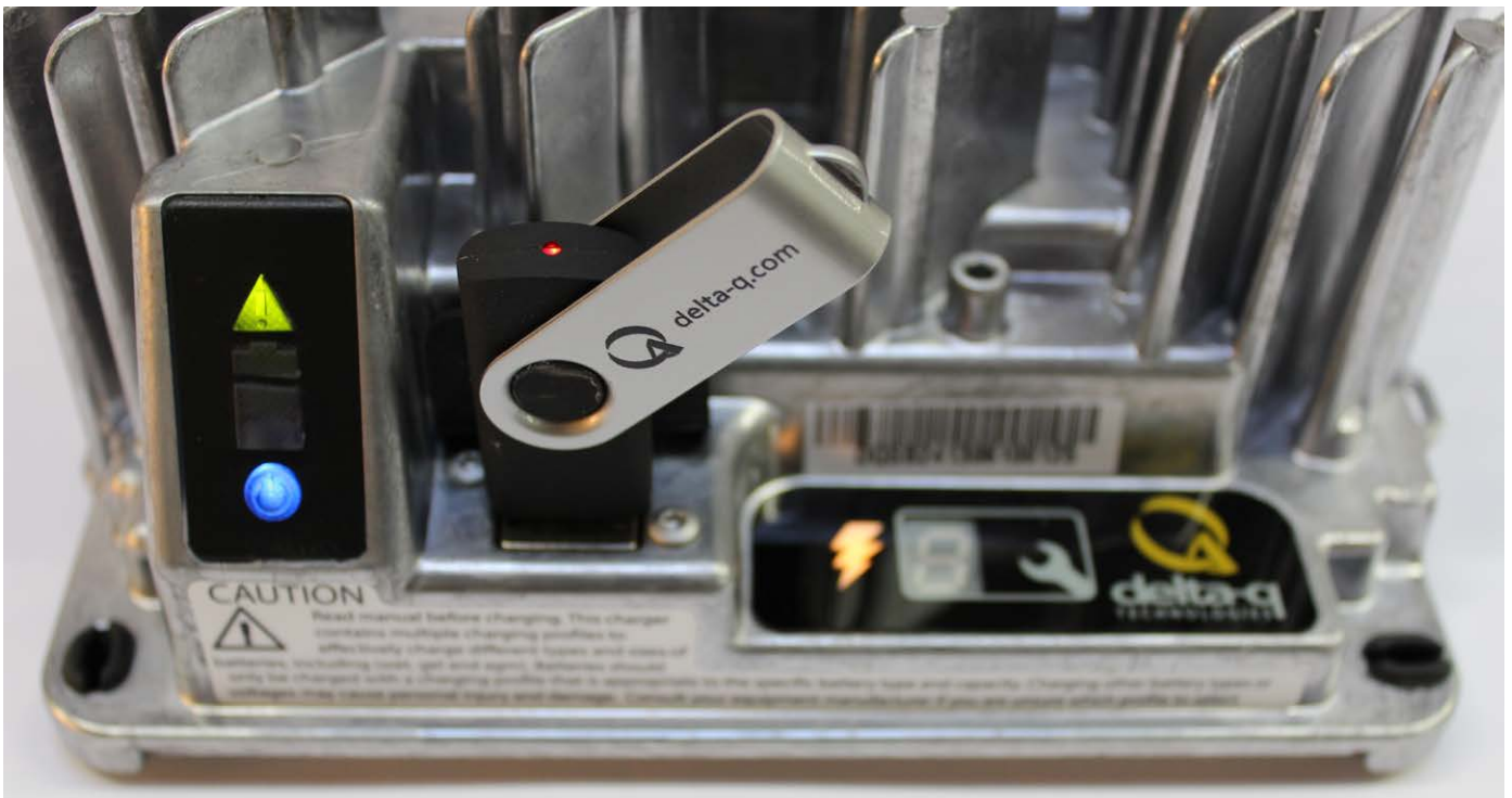
Figure 31. Insert the USB flash drive to begin the charge data download process. This step can be completed using the same USB flash drive programmed to update the charger's software. The process is completed when the USB indicator is solid green, and no longer flashing.
