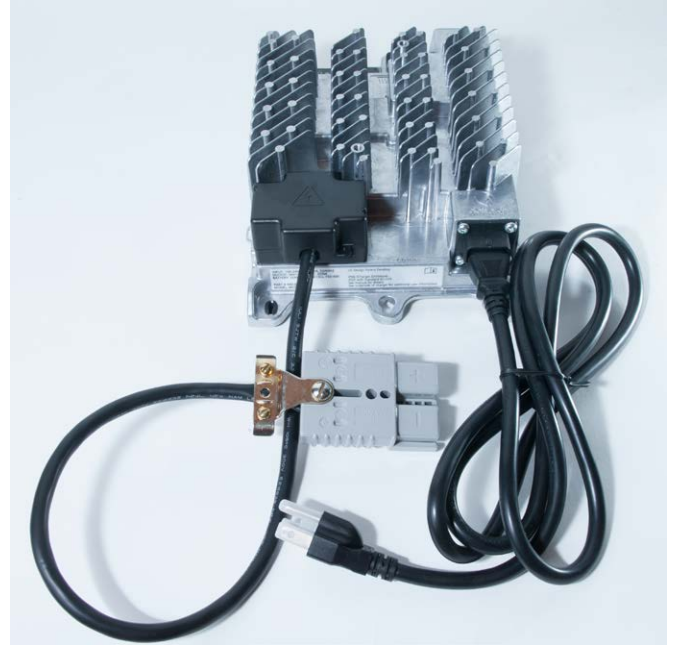
Figure 18. Both the DC and AC cabling has been installed on this IC650 Charger. Using cable ties with the AC cabling is recommended, as these cables may be pulled out of the mating connector.
