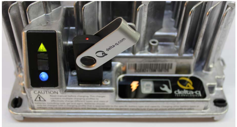
Figure 30. Insert the USB flash drive to begin the reprogramming process. When complete, the Fault / Error / USB indicator will be solid green as shown.
